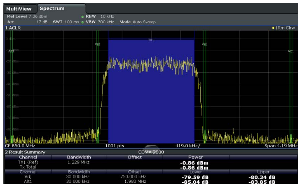
Fig. 4-5: Adjacent channel power measurement on a CDMA2000 1x signal
